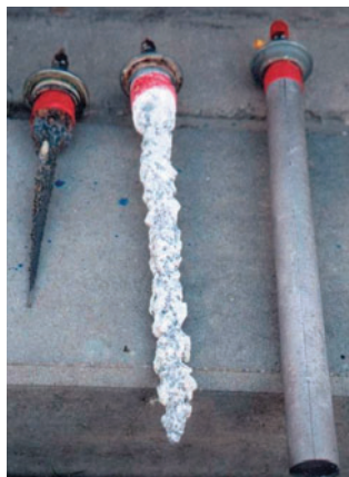
Magnesium anode bar used in hot water tanks
